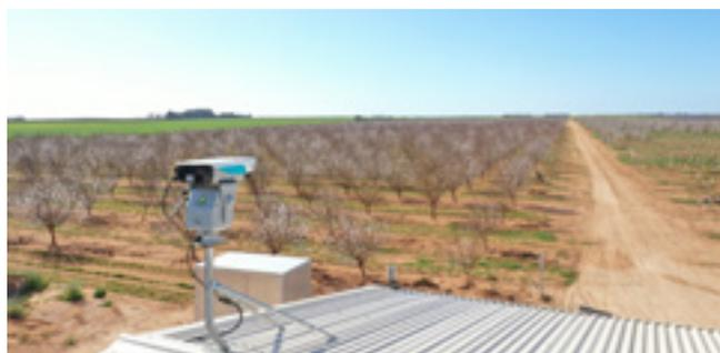
Figure 3. Bird scaring laser
